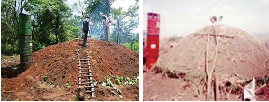
Figure 6: Typical Casamance kiln in Senegal (left) and Ethiopia (right)
